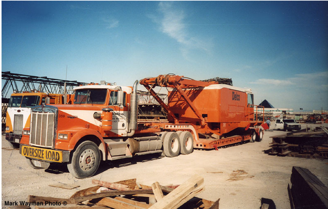
AMERICAN 9310 CRAWLER CRANE, 225 TON, W/O CAR BODY ON 5 AXLE LOWBOY
