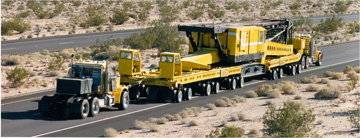
AMERICAN 11320 CRAWLER CRANE, 450 TON, HOUSE, CAR BODY & BUTT SECTION ON A 13 AXLE TRAILER
