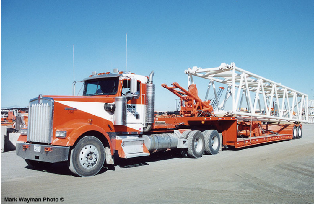
CENTER DROP TRAILER WITH CWT. & BOOM
