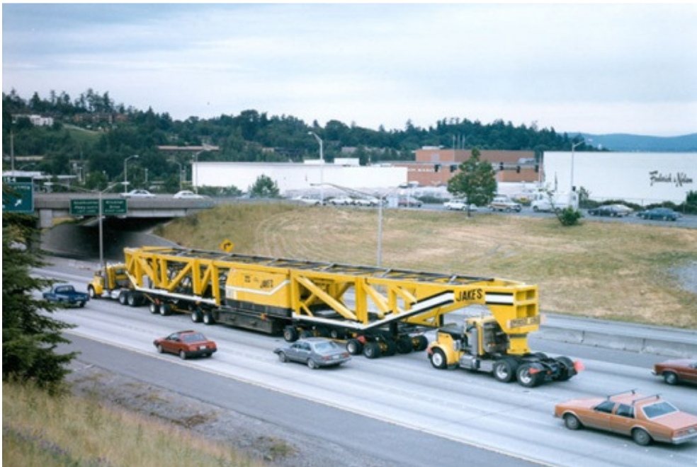
AMERICAN 11320 CRAWLER CRANE, 450 TON, HOUSE, CAR BODY & BUTT SECTION ON A 16 AXLE TRAILER
