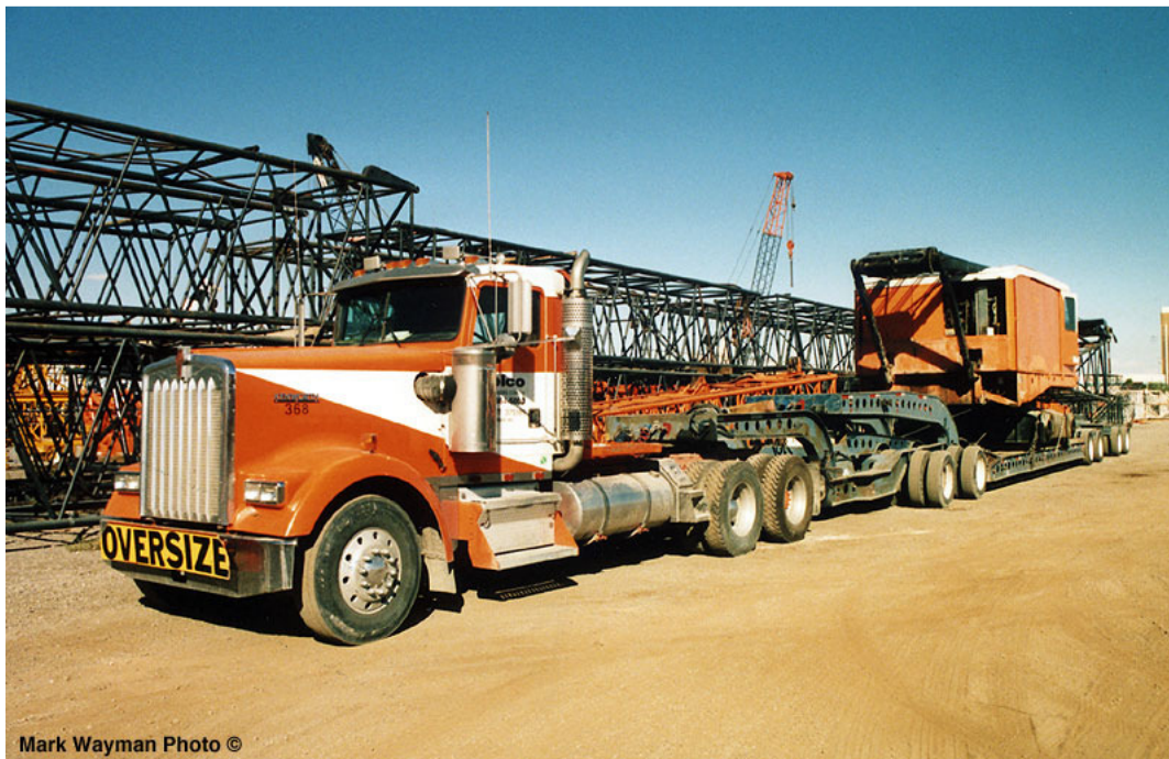
AMERICAN 9310 CRAWLER 225 TON W/HOUSE & CAR BODY ON 9 AXLE TRAILER
