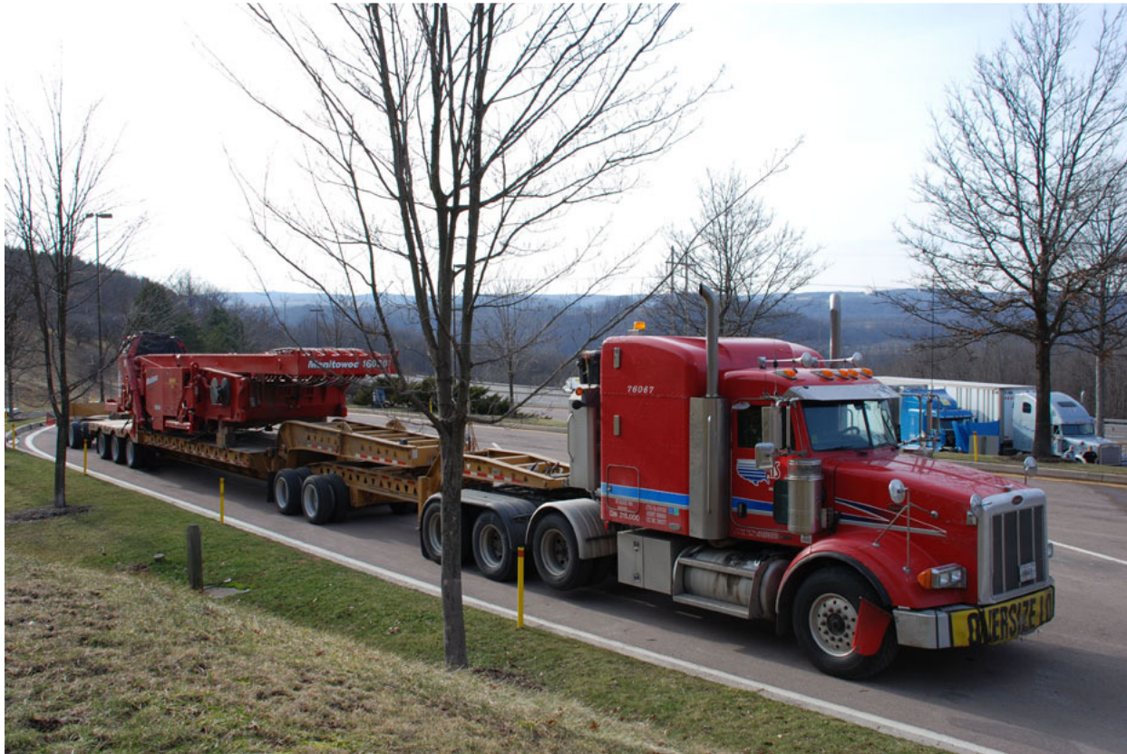
MANITOWOC 16000 CRAWLER, 440 TON, HOUSE BEING TRANSPORTED ON A 11 AXLE LOWBOY
